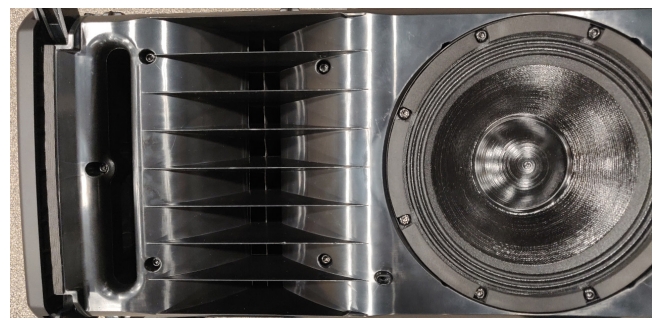
Figure 1. Close-up of the QSC LEAF™ waveguide in the LA108 active line array loudspeaker.
